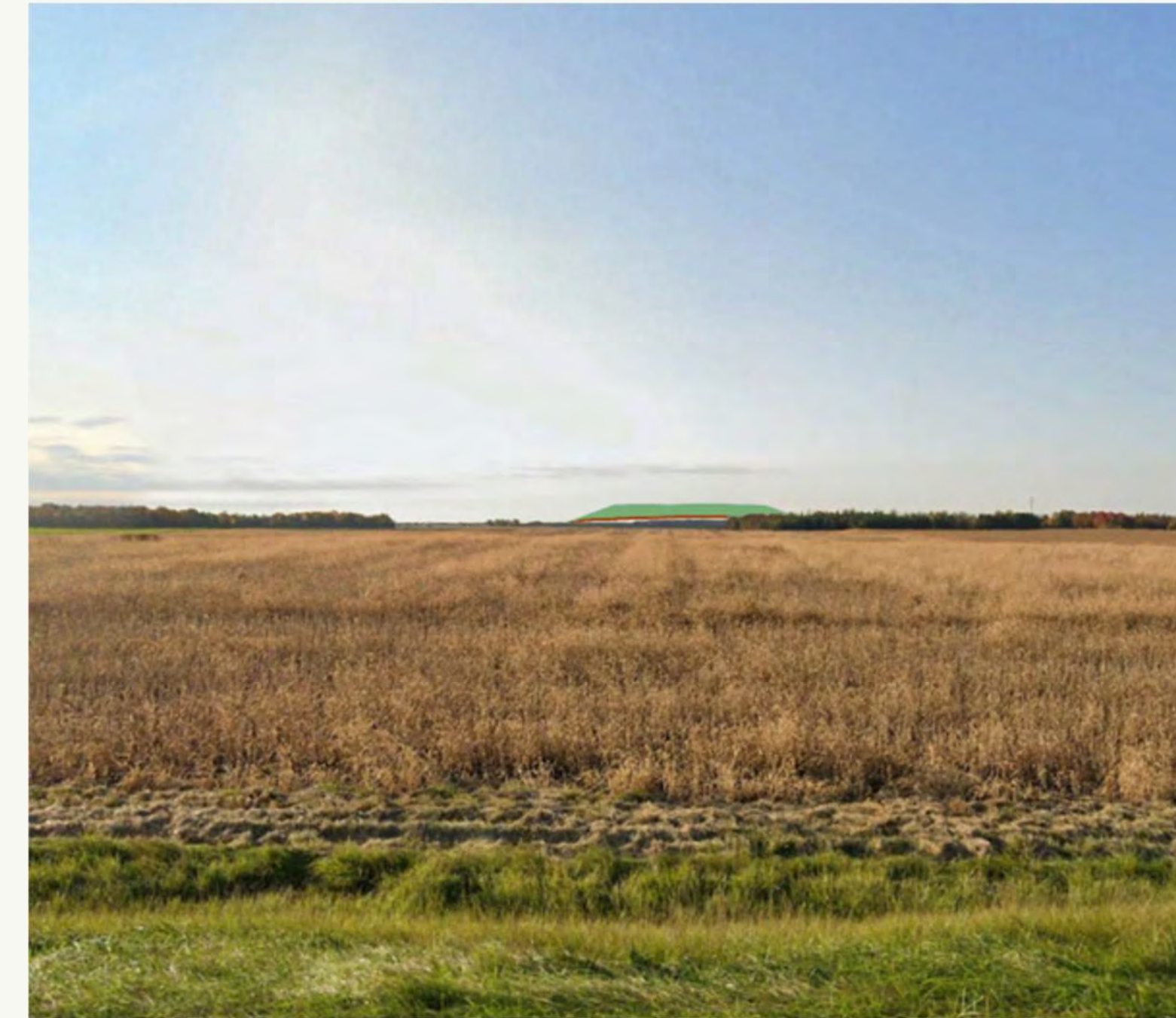
Viewpoint 6 Visible Landfill Area = 19,228 m 2 , index 6.8; effect value = 1. Distance = 2,820 m; effect value = 1. Horizontal Angle of View = 11°; effect value = 1. VACF = 1; effect value = 5. CEV = 8; low effect.
