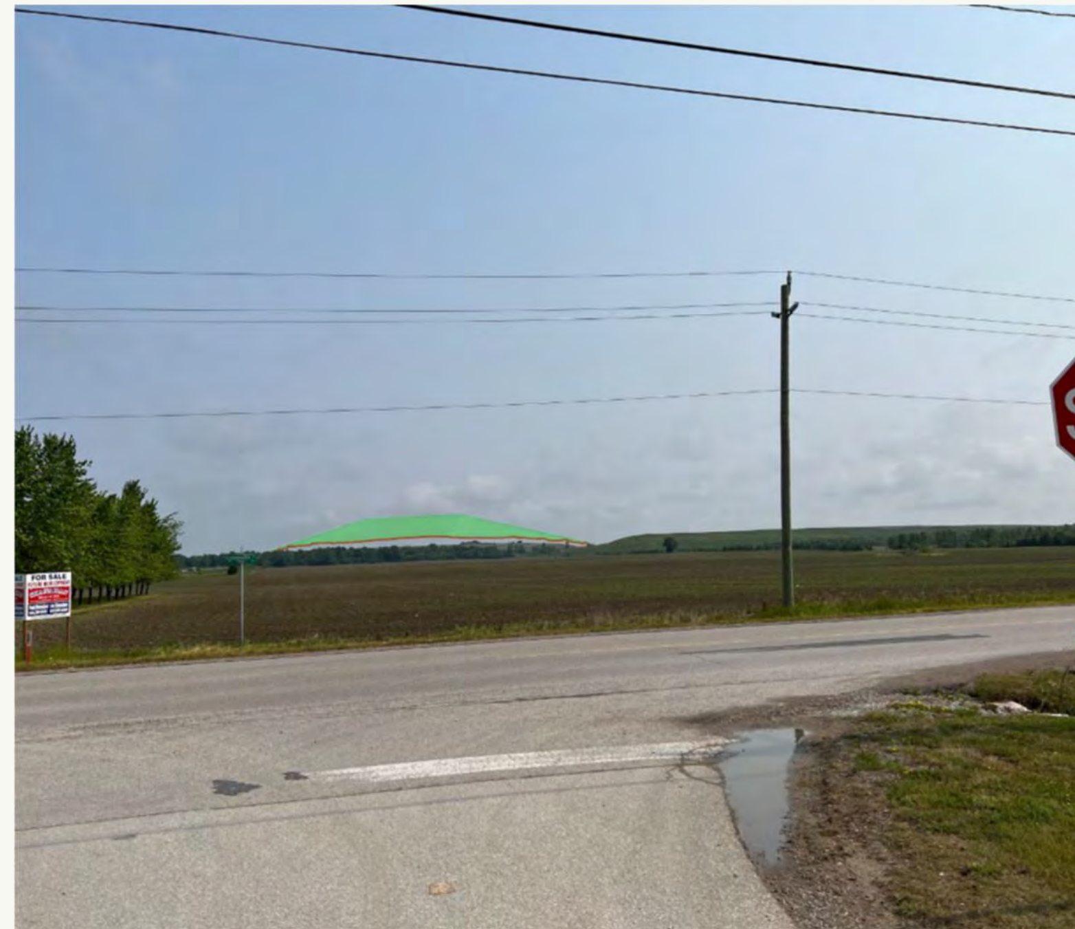
Viewpoint 4 Visible Landfill Area = 20,949 m 2 , index 15.1; effect value = 3. Distance = 1,387 m; effect value = 3. Horizontal Angle of View = 14°; effect value = 1. VACF = 1; effect value = 5. CEV = 12; moderate effect.
